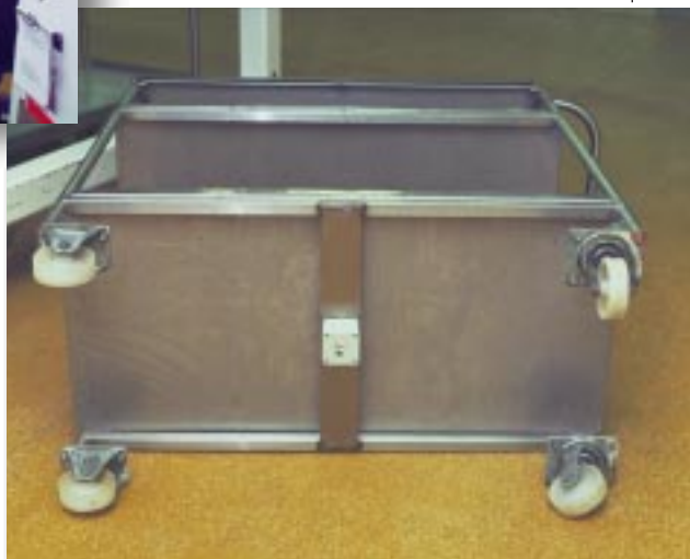
Tag with unique ID attached to bottom of stainless steel cart for automatic product tracking.
